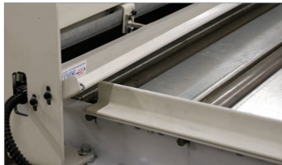
Special HPL cleaner with ionization unit, brush and vacuum pump
